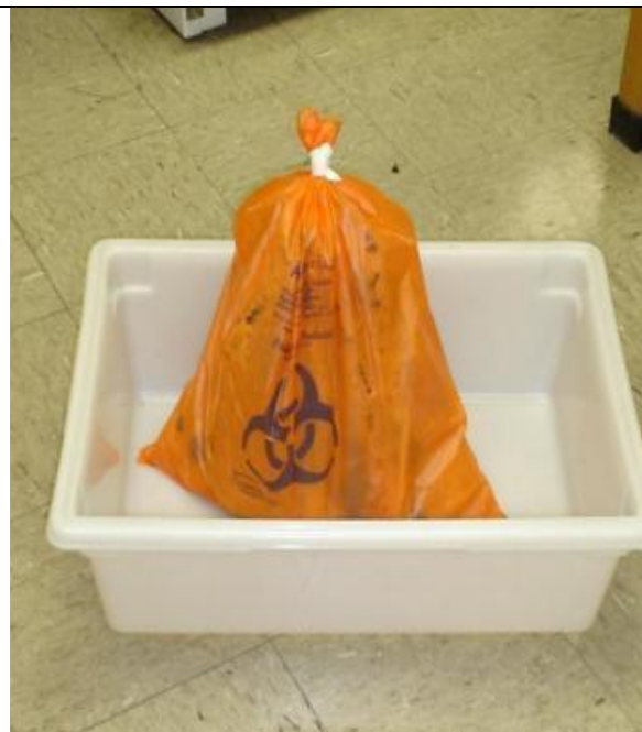
Biohazardous waste bags awaiting treatment should always be stored in pans or secondary containment to prevent spills!
